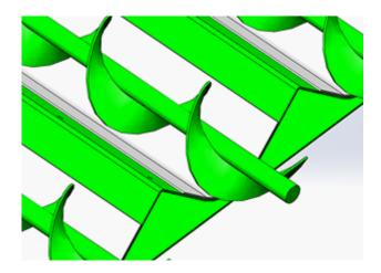
**Step 3** - Use shims (if required) to hold liner down tight against auger bed floor.
