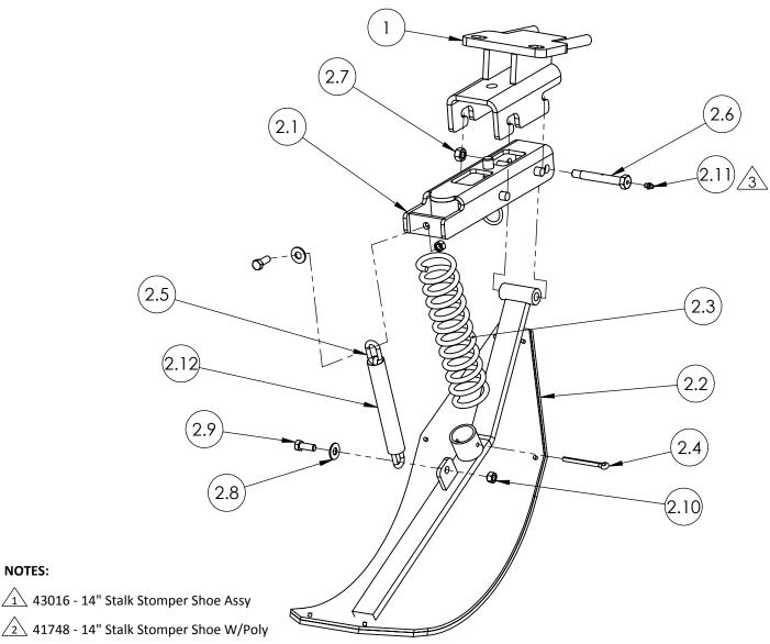
Install Self-Tapping Grease Fitting into end of Pivot Bolt Torque grease fitting to 65-70 inch pounds. DO NOT OVERTIGHTEN!
