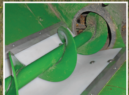
AUGER TROUGH & FLOOR LINERS
